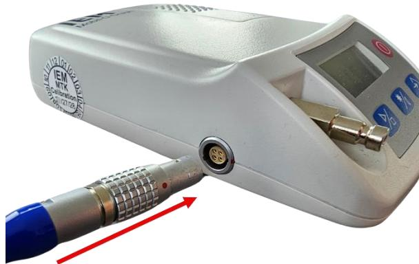
Do not attempt to force the download cable as this can cause damage to both the cable and the device.
