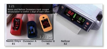
Three finger pulse oximeters and one tabletop pulse oximeter were attached to a subject who was breathing for the first minute using a commercially available rebreather\* to induce hypoxia.
