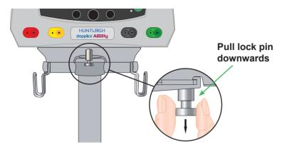
Release the lock pin and ensure it locates in the hole in the mounting plate. This can be verified by attempting to slide the Ability unit sideways. It must be securely locked into position.
