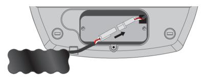
3. Replace the battery. Re-fit the battery cover and replace the securing screw with the allen key provided. **DO NOT OVERTIGHTEN!**
