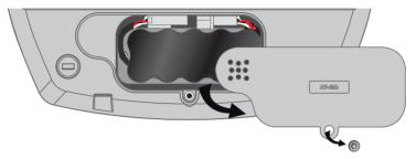
2. Lift the battery out, and connect the battery to the unit.
